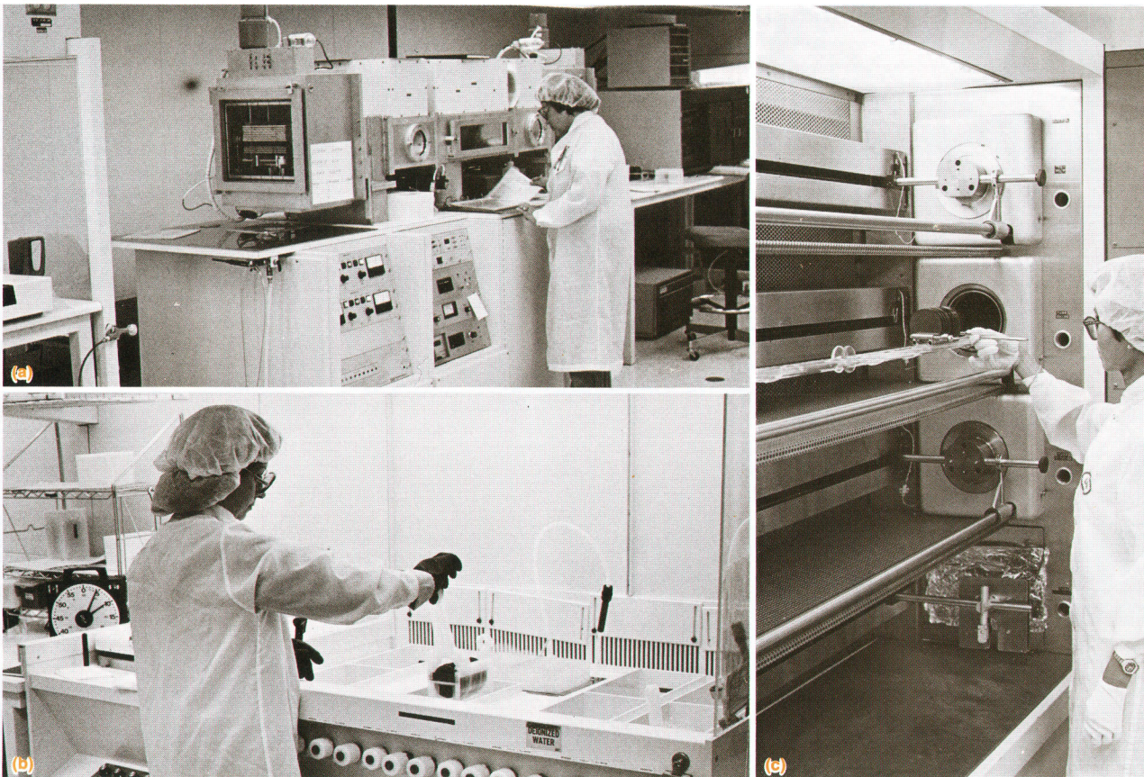
Fig. 1. (a) Planar magnetron system used for metal deposition. (b) One of the wafer etching and cleaning benches. (c) Loading wafers into low-pressure chemical-vapor-deposition (LPCVD) system.
