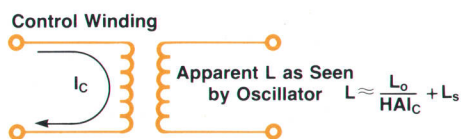
Fig. 7. Simplified schematic of the variable control inductor shown in Fig. 5.
